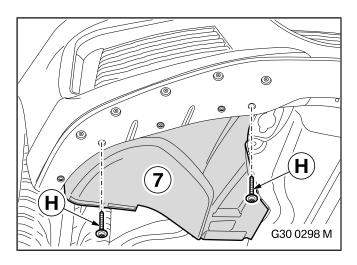
Install the air guide (7) with screws **H**.
