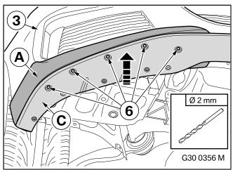
The holes must be drilled through the "right front attachment, carbon" **A**, "left front attachment, carbon" **B** and the bumper support (3). When drilling down to the drill depth, take care not to damage parts underneath. ◀
