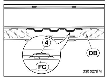
Install the clips **FC** on the lugs (4) using a suitable tool.
