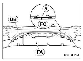
Insert the "Carbon rear diffuser" **FA** with lugs (5) into the "Matt black rear bumper trim" **DB**.
