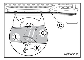
Install the "Carbon front add-on section" **C** using Alan screws **K** and washers **L**.
