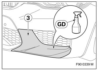
The bonding surfaces must be completely dry, clean, and free from wax or grease. ◀
