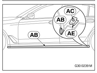
Install sheet metal nut **AE** using oval-head self-tapping screw **AC** on "Matt black side sill add-on section, left" **AB**.
