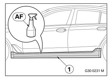
The bonding surfaces must be completely dry, clean and free from wax or grease. ◀
