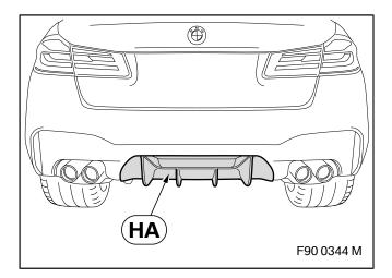
Remove standard installed rear diffuser as described in **ISTA/AIR**.
