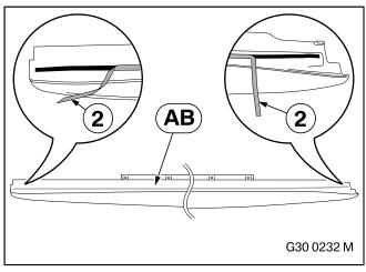
Release a little of the adhesive backing film (2) on both sides of the "Matt black side sill add-on section, left" **AB**.
