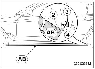
Ensure that the released ends of the adhesive backing film (2) are visible. ◀
