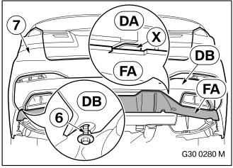
Insert the assembly of "Matt black rear bumper trim" **DB** and "Carbon rear diffuser" **FA** in the rear trim (7) so that the four lugs **X** are completely inserted in the "Exhaust system support adapter cover" **DA**.
