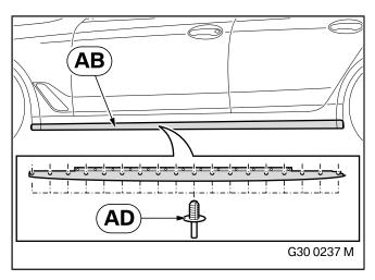
Install the "Matt black side sill add-on section, left" **AB** using expanding rivets **AD**.
