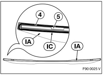
Sand and clean the edge area (4) of the "Carbon Pro rear spoiler" **IA** using suitable tools.
