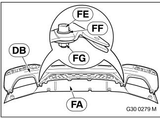
Secure "Carbon rear diffuser" **FA** at the left and right using ISA screws **FE**, washers **FF** and hexagon nuts with washer **FG** to the "Matt black rear bumper trim" **DB**.
