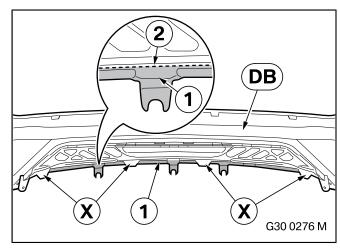
Ensure that the four lugs **X** are not removed from the "Matt black rear bumper trim" **DB**. ◀ Cut the flange (1) along the cutting line (2) using a suitable tool.
