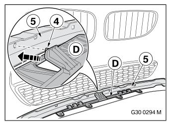
Insert the "Adapter front top" **D** with bolt (4) in the direction indicated by the arrow in the cross member (5).
