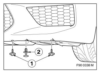
Remove screws (1) and clip (2) as described in **ISTA/AIR**.
