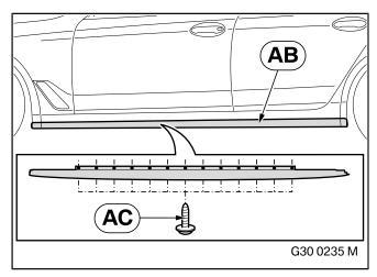
Install the "Matt black side sill add-on section, left" **AB** using oval-head self-tapping screws **AC**.
