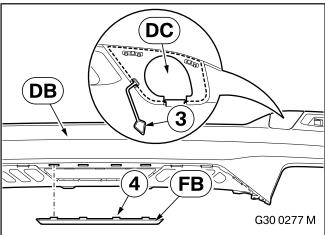
Insert the "Towing eyelet cover" **DC** with retaining hook (3) into the "Matt black rear bumper trim" **DB** as shown.
