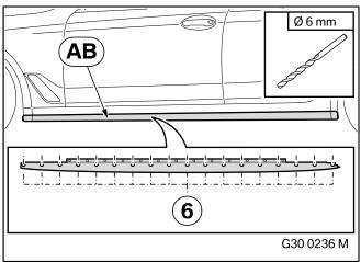
When drilling down to the drill depth, take care not to damage parts underneath. ◀
