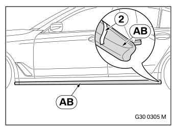
Carefully remove the adhesive backing film (2) from the outside inwards and firmly press on the "Matt black side sill add-on section, left" **AB**.
