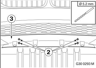
When drilling down to the drill depth, take care not to damage parts underneath. ◀
