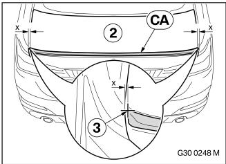
Position the "Matt black rear spoiler" **CA** on the marks (2) you made earlier on the boot lid (2), centre it and mark the position (3) with suitable tools.
