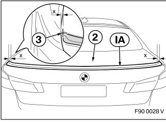
Position the "Carbon Pro rear spoiler" **IA** on the boot lid (2), centre it and mark the position (3) with suitable tools.
