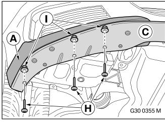
Align the "front attachment, carbon" **C** and install it with screws **H** and plastic cap nuts with washers **I**. Ensure that the gaps to the "right front attachment, carbon" **A** and "left front attachment, carbon" **B** are uniform.
