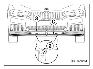
Mark the fastening points (2) for the "Carbon front add-on section"  $\bf C$  on the bumper support (3) using suitable tools (4x).
