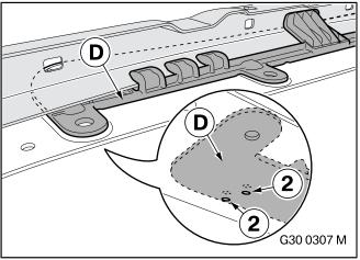
Align the "Adapter front top" **D** with the fastening points (2).
